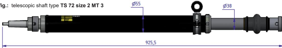
fig.: telescopic shaft type TS 72 size 3 MT 3
