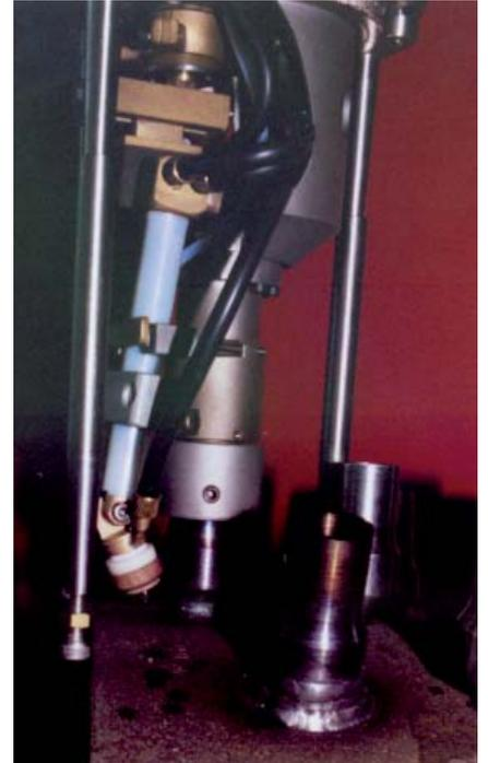
special torch for header drum stud welding
