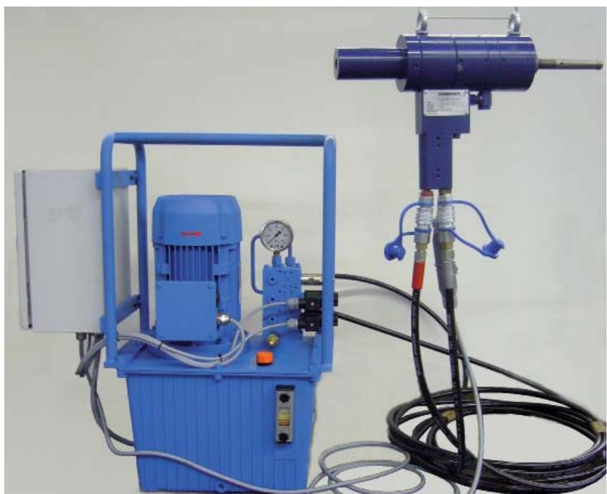
**Tools for mechanical-hydraulic tube contact expanding Type TES 97**
